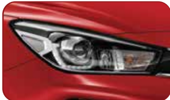
Bi Function Headlamp with LED DRL & Static Bending Light
